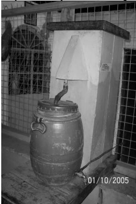
Figure 14 BSF with Safe Storage from Machakos, Kenya (Baffrey, 2005)
